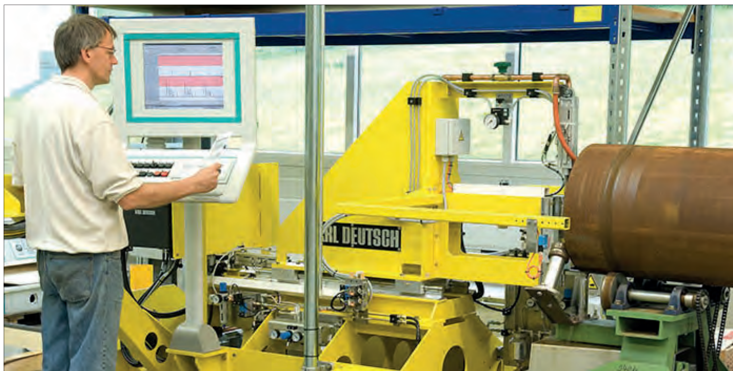
Entering the test parameters and checking the calibration of the test system
