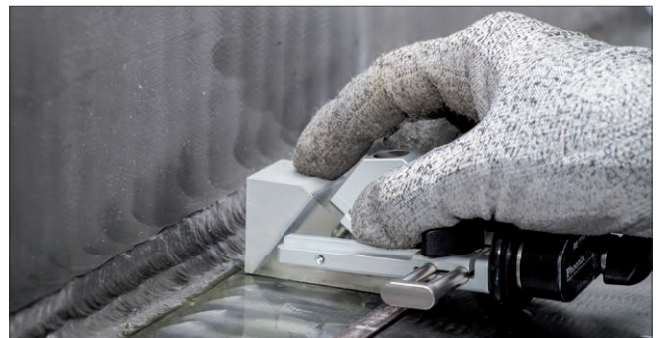
Ideal field of application for the MANTIS: The imaging test on a fillet weld
