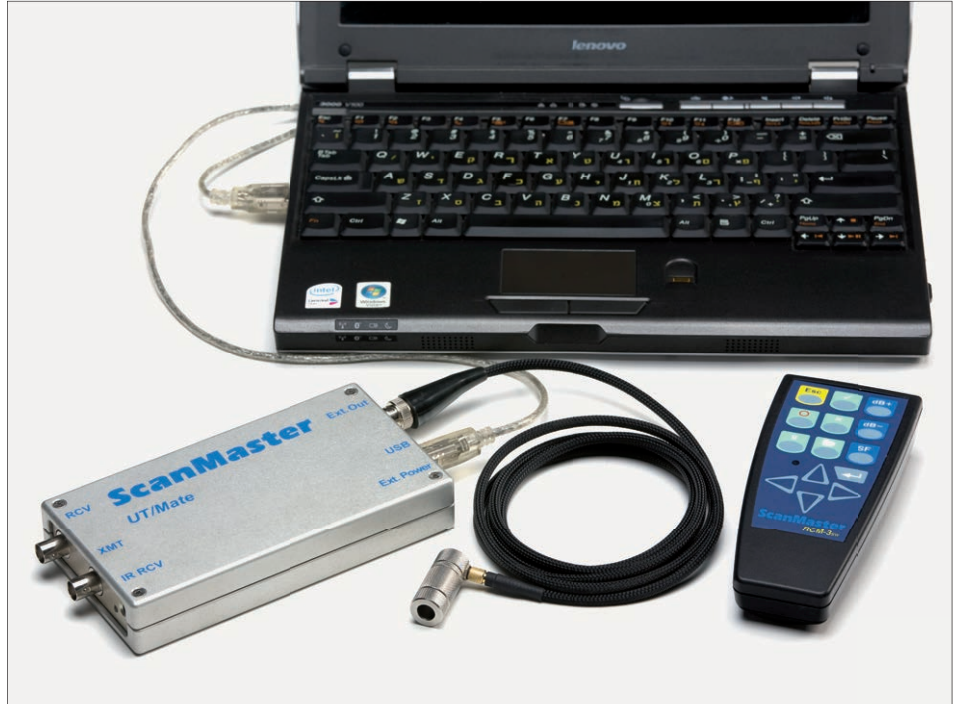
Fig. 4: Laptop with ScanMaster module UT/Mate, probe and remote control
