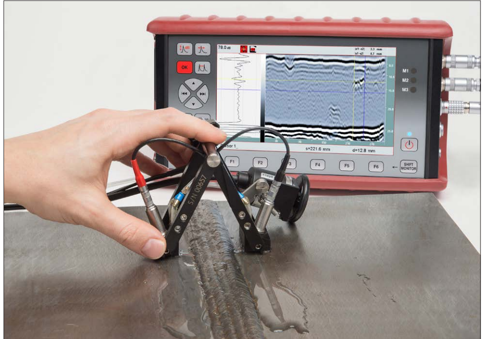
Fig. 3: ECHOGRAPH 1095 during TOFT testing with scanning device
