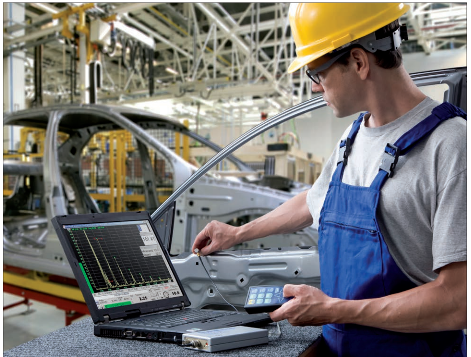
Fig. 1: Examination of spot welds in the car body making industry
