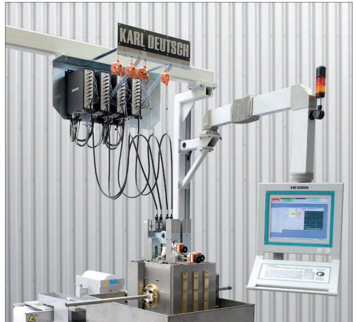
Fig. 1: ECHOGRAPH-HRPR tube testing system with immersion tank and ultrasonic pre-amplifiers above the tank
