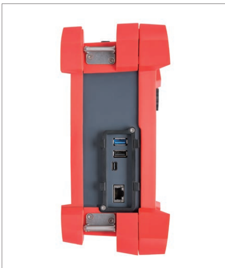
The lateral standard interfaces of the MANTIS: USB and LAN
