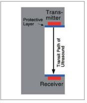
Principle sketch of the special probe: Transmitter and receiver units are covered with a protective layer which is short-time resistant against aggressive outside influences
