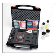
Delivery in a handy carrying case containing the probe, PC software tool **KonzBest**, temperature meter **Check-temp**, 250 ml fully desalinated water, two beekers and the instruction manual
