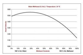
The interdependency of concentration and sound velocity using the example of the mixture Methanol and water
