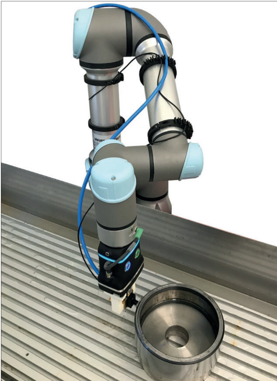
Test setup with horizontal ring for automatic vertical alignment of the probe
