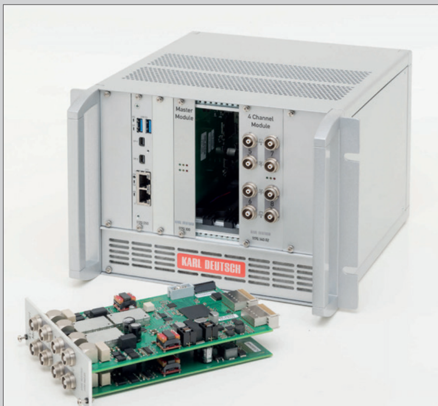
The ECHOGRAPH 1170 testing electronics is based on very compact, four-channel modules that are interconnected according to the number of channels. Since special through-transmission methods are also supported (e.g. for nodularity testing on castings), eight LEMO sockets can be seen.
