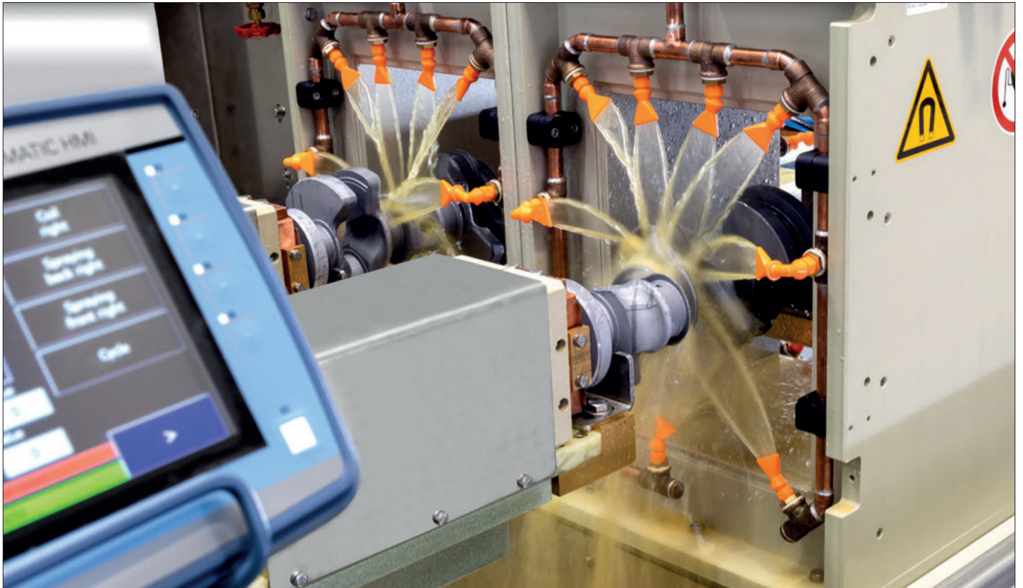
DEUTROFLUX UWS dual station for fast crankshaft testing with moving coil
