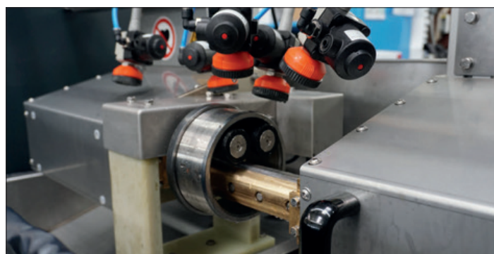
Magnetising unit for ring testing with decentralised mandrel
