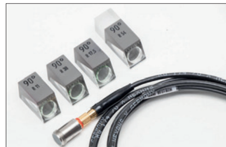
Different probes for different materials of the pipelines to be examined
