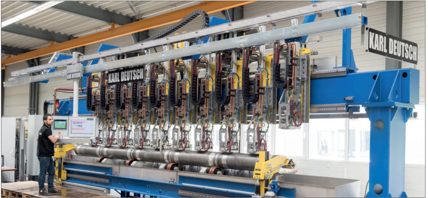
ECHOGRAPH ALPT test bridge for aluminium round bars with eight test systems
