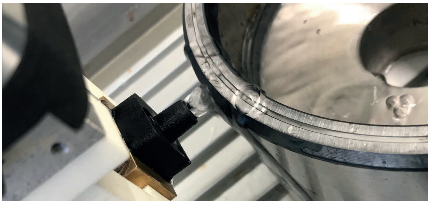
Water nozzle coupling for bearing ring testing with a robot
