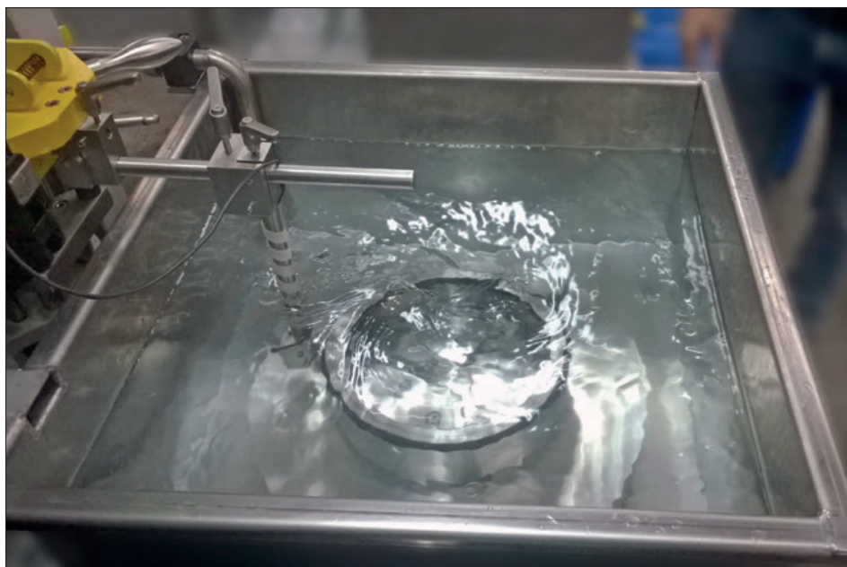
View of the rotating ring at maximum test speed
