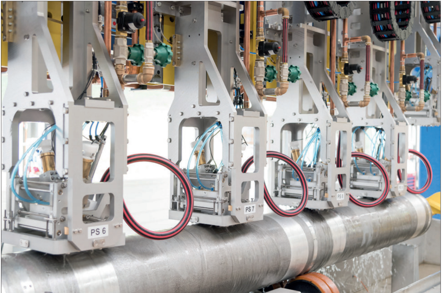
Cardanically suspended testing systems, each with one vertical probe and two angle probes
