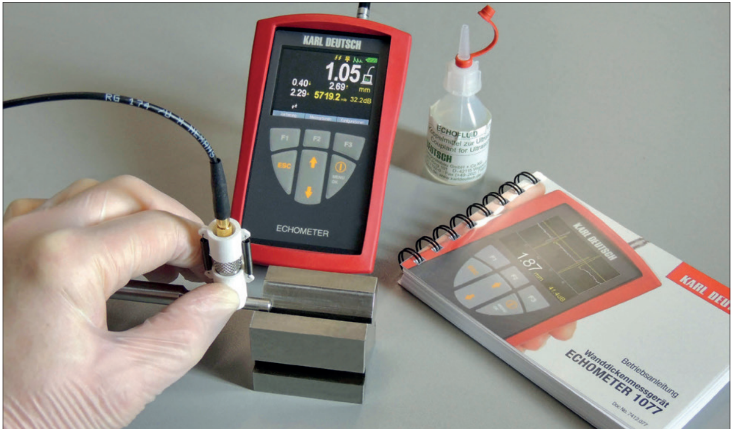
Wall thickness measurement of a metallic protective sleeve at several circumferential points to assess the eccentricity
