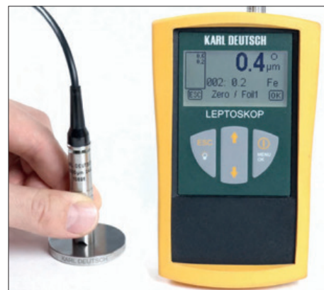
Calibrating the LEPTOSKOP 2042
