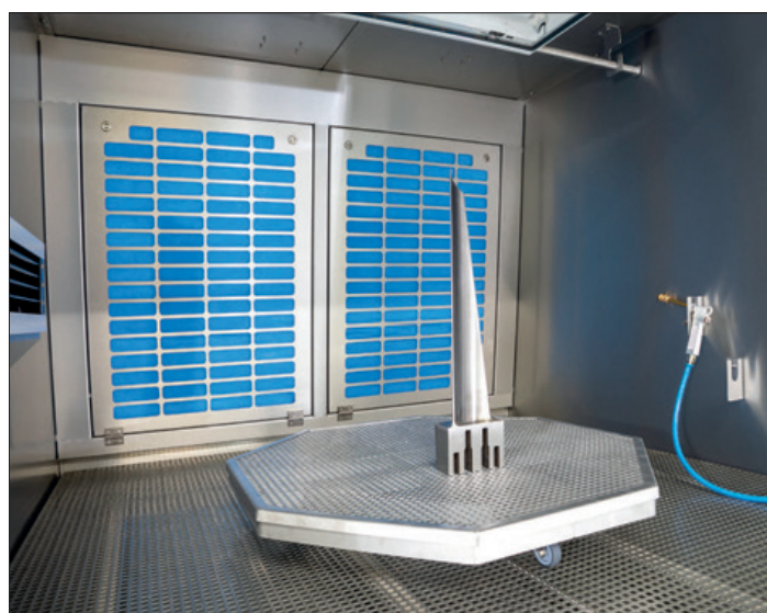
Test chamber with turntable and internal connections for water and compressed air (with a laboratory test part)
