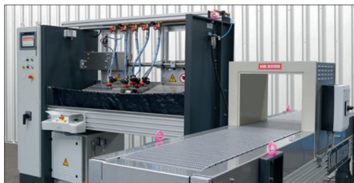
Conveyor belt with integrated ESV demagnetising coil
